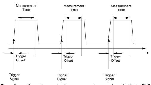
Depending on the settings made, the measurements are performed with the RMS detector for RMS power or the PEAK detector for peak power. For all these measurements, TRACE 1 of the selected system is used.
